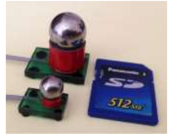
Fig 6. 3-axis piezoelectric actuators based on radial resonant travelling wave oscillations.
